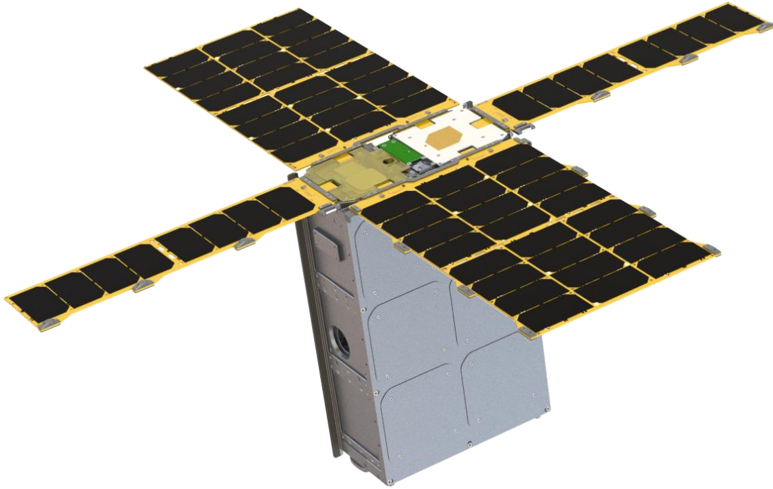
Figure 15-7: Pumpkin Inc.'s 6U SUPERNOVA bus
