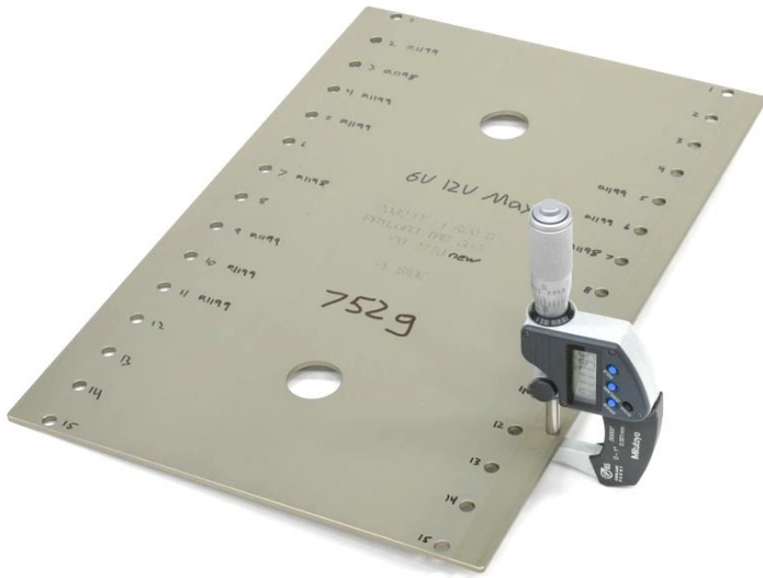
Figure 11-3: Measuring tab thickness with micrometer
